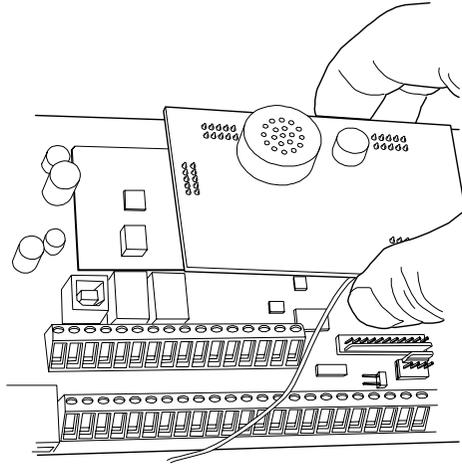
Figure 5. Fitting i-gsm02 Module
