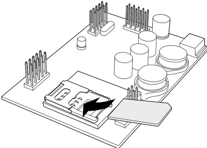
Figure 4. Fit a SIM Card
